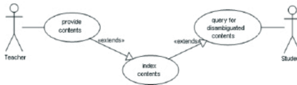
Fig. 1 - Use case UML Diagrams of the proposed system the two actors interfacing with the systems are the teacher and the student.
