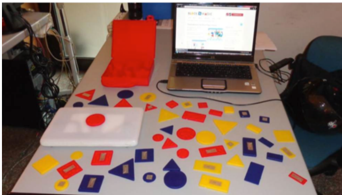
Fig. 3 - The Block Magic prototype that includes a tablet able to recognize each RFID tag and transmits the signal to the PC/tablet; a tablet equipped with a dedicated software and enhanced with Artificial Intelligence; 48 Logical Blocks tagged with RFID antennas
